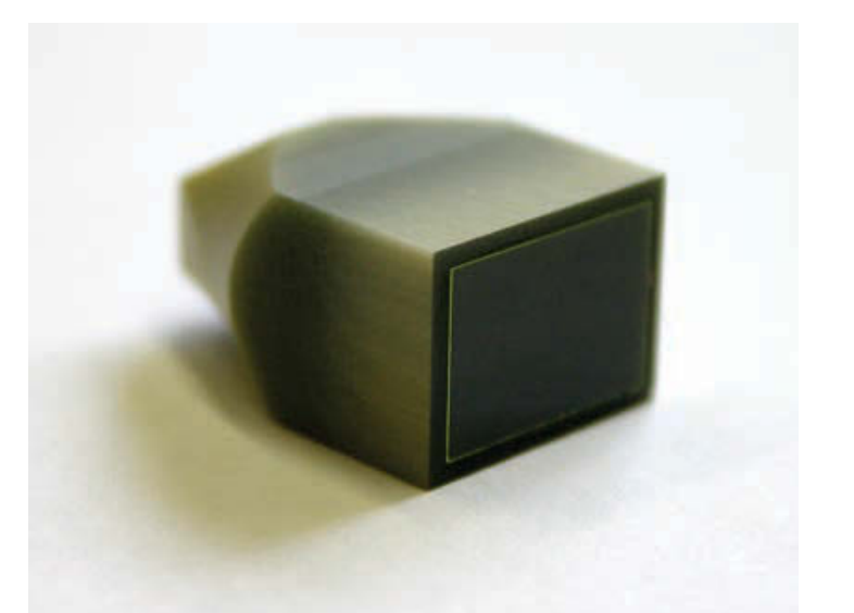
Thin YAG:Ce Screen on FOP
