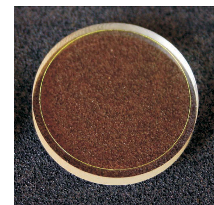
5 \mu m Thin YAG:Ce Screen
